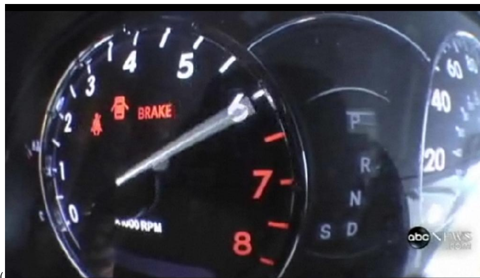
Figure 3. High engine speed resulting from signal manipulations, ABC Video at 2:15.
