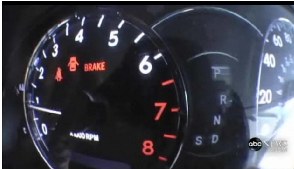
Figure 2. Idle speed condition of the vehicle prior to connecting the power supply to the resistor, ABC video at 2:15.
